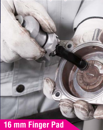
Removing burrs on the castings around the spot where the ejector pin contacts
