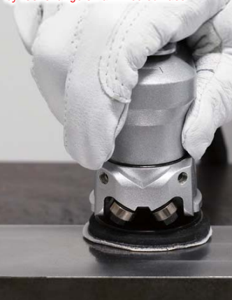
Sanding a slight difference in level caused by tool change on a milled surface
