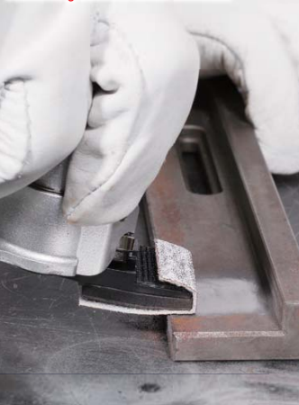
Removing rust on small surfaces
