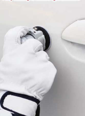
Putty sanding to remove light scratches
