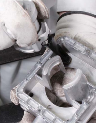
Removing burrs on confined areas of the casting
